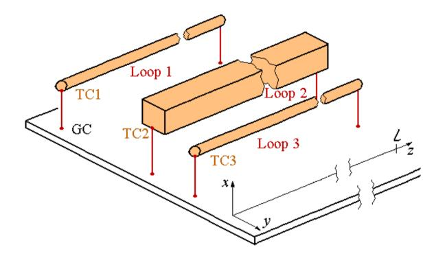
□ For a (n + 1)-conductor uniform MTL, for a uniform current distribution and for L >> transverse dimensions,  $L_{DC}$  is nearly proportional to L. The p.u.l. inductance matrix is
